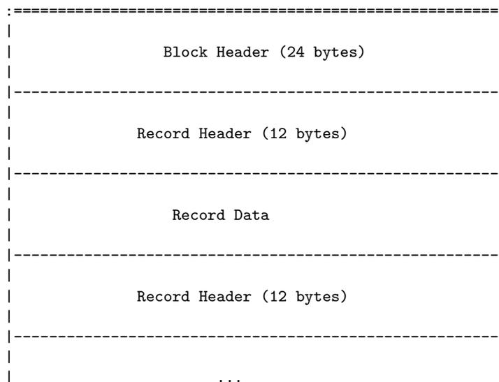
Block Header: the first item in each block. The format is shown below.
